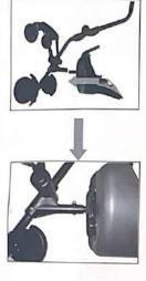
6. Assembly of the steering-wheel handle: Connect the handle with handle post and fasten with the M6 screw and M6 nut.Please make sure it is securely tightened before use.
