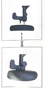
4. Install and removal of the rear wheel: Insert the wheel pin to the rear wheel housing until it clicks to install the wheel, gently pull it to ensure it's firmly installed. Make sure both back wheels are assembled correctly before use. Pull up the pin on the back axel to remove the wheel from the rear housing.
